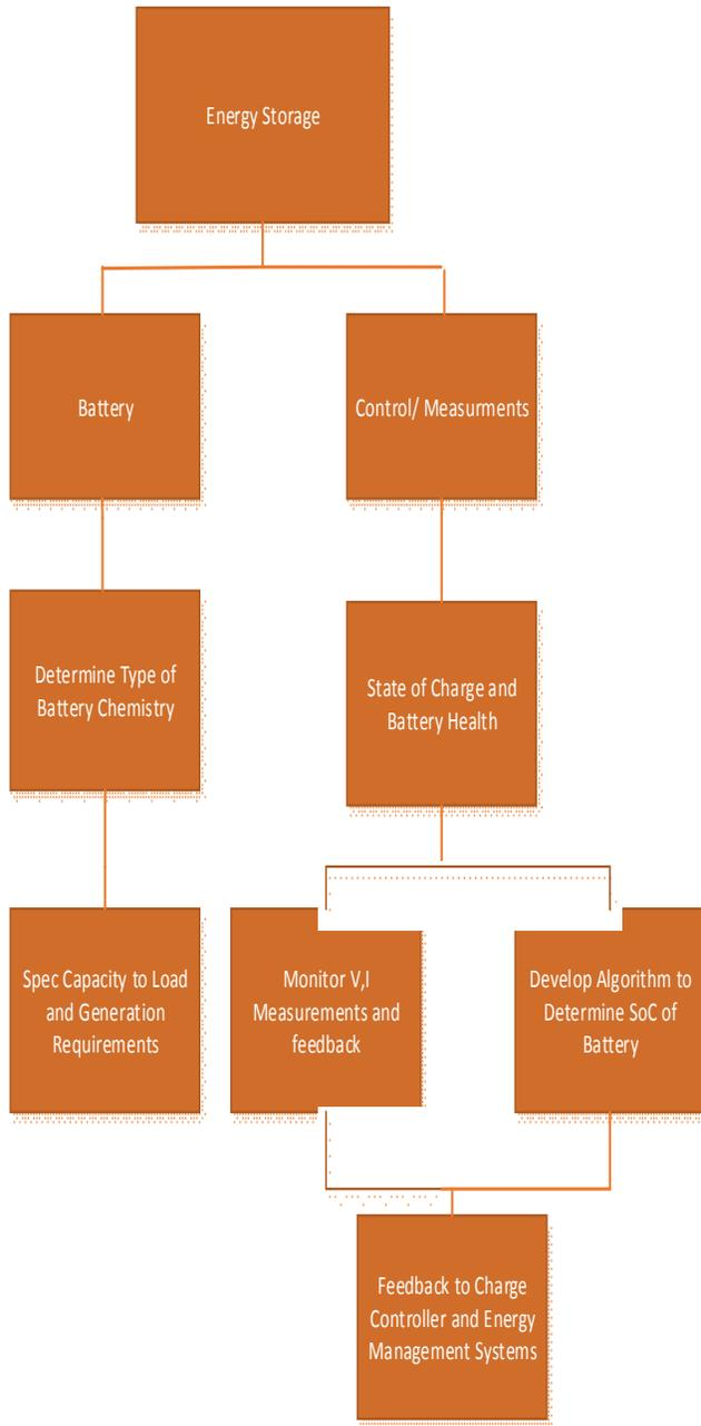
Figure 13: WBS Flow of the Energy Storage Stage
