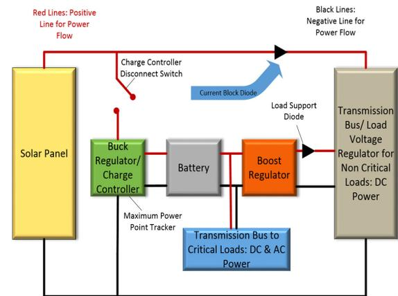
Figure 35: Block Diagram of Microgrid Power Flow
