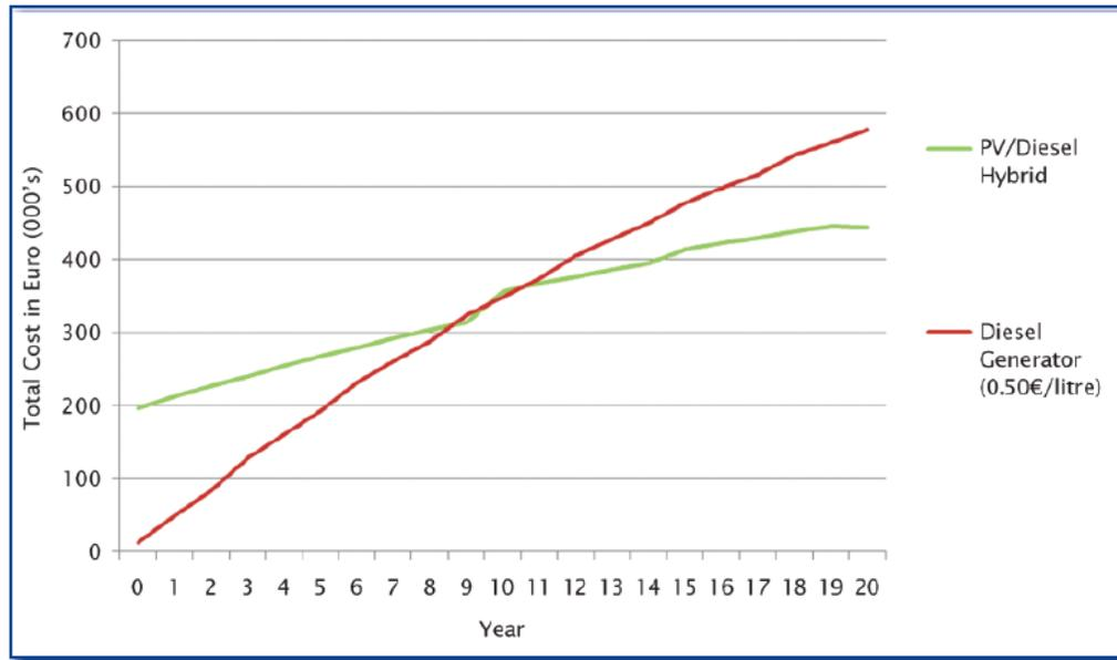
Figure 27: Cost over time of PV microgrids and Diesel microgrids.
